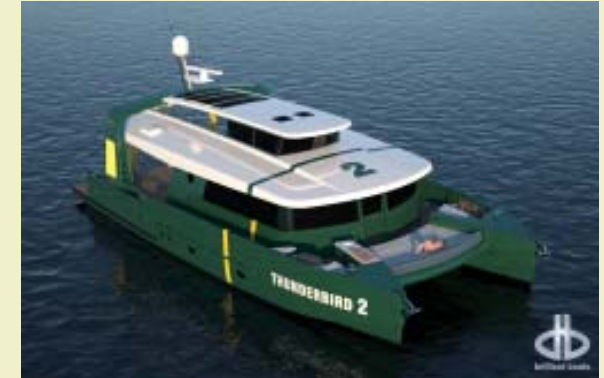
The Triton 65' catamaran carries a Triton on a platform aft between the hulls that is lowered into the water to launch and recover the sub.
