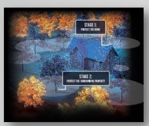
Stage One, FireIce powder is combined with water pumped from an underground storage tank. This creates the FireIce protective gel, a revolutionary fire retardant product used by many professional firefighting organizations to stop fires fast. Multiple fire suppression lines installed on the home deliver the FireIce gel so that it covers the home. As the fire nears, the control panel activates Stage Two.
