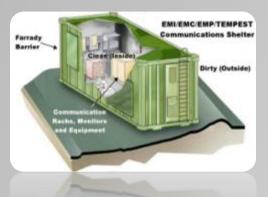
reduce the coupling of EMP electric and magnetic fields into the protected area. The electromagnetic barrier shall consist of the Facility HEMP Shield and protective devices for all POE's. Additionally, reliability, maintainability, safety and human engineering, testability, configuration management and corrosion control all need to be incorporated to the HEMP protection system design.
